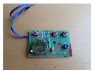
Front of remote control circuit board, showing three switches and battery.
