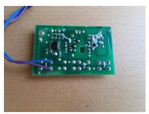
Back of remote control circuit board with wires soldered to the momentary switch
