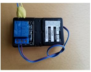
Back of remote with the case replaced, the relay module and wires attached.
